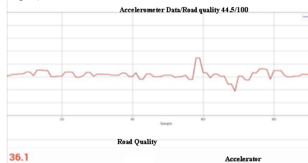
Figure 5 Road quality measured using an accelerometer
