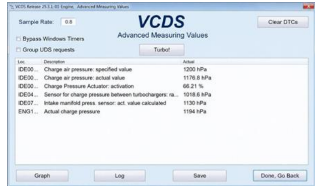
Figure 3 MAP parameter values under load at approximately 2600 rpm
