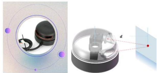
Figure 9 LiDAR – operating principle. [6]
