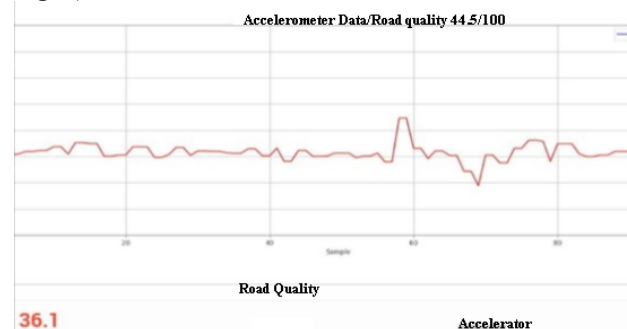
Figure 5 Road quality measured using an accelerometer
