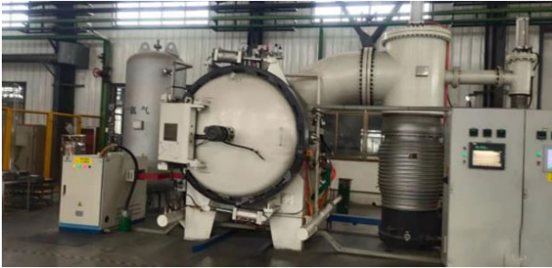
Figure 6 Vacuum annealing treatment [15]
