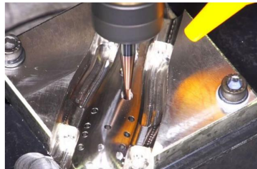
Figure 3 Cutting and Machining Moulds
