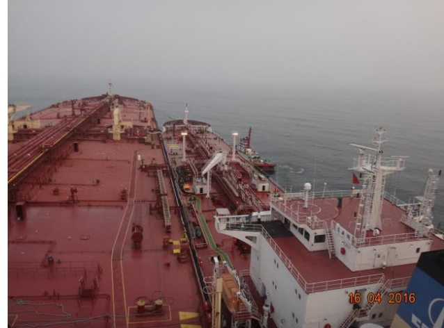
Figure 2 VLCC during Ship To Ship crude oil transfer operation to a Panamax size vessel in the Gulf of Tonkin (Source: Author's personal archive).
