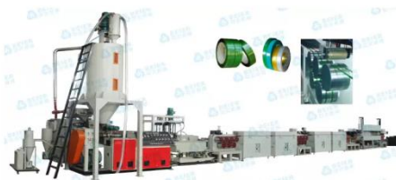
Figure 2 PET strap production line [6]
