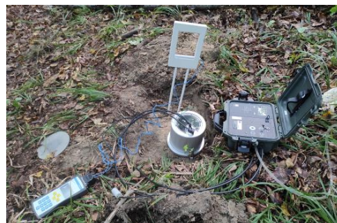
Figure 6 Measurement by the EIS system with a mobile fork probe and the Z-meter IV device, including the use of a control device SATURO
