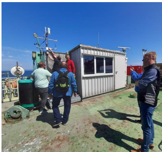
Figure 11. Testing the position of the wind, pressure, precipitation, solar radiation sensor system (photo)
