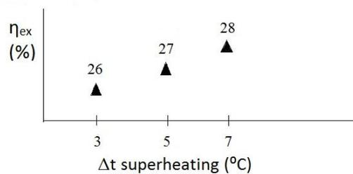
Figure 5 Exergy efficiency versus superheating degree
