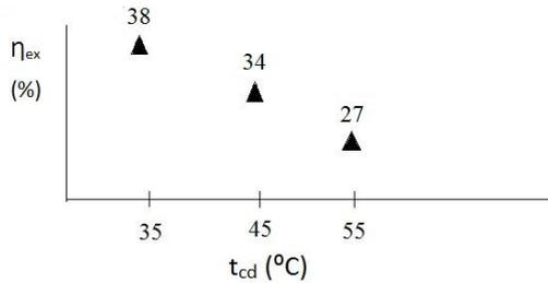
Figure 3 Exergy efficiency versus condensation temperature (evaporation temperature is kept constant)
