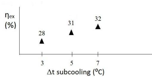
Figure 7 Exergy efficiency versus sub cooling
