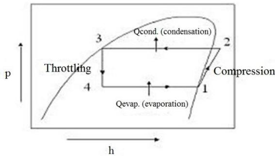
Figure 1 Vapour compression refrigeration cycle without sub cooling and superheating in (p-h) diagram.
