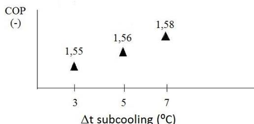
Figure 6 COP versus sub cooling degree
