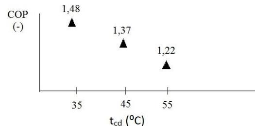
Figure 2 COP versus condensation temperature (evaporation temperature is kept constant)
