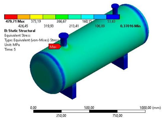
Figure 4 The state of tension in the equipment
