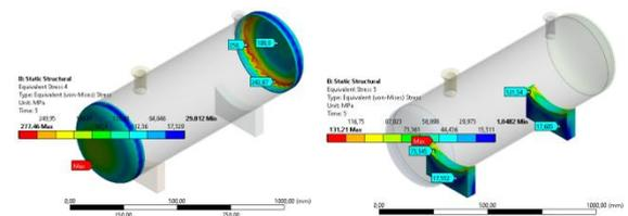
Figure 6 The state of tension in the jacket and connections
