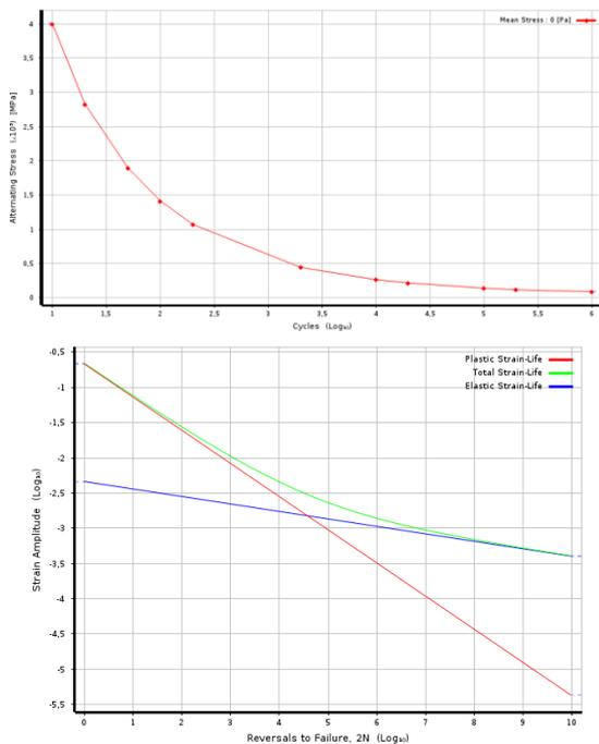
Figure 6 Wöhler theoretical diagram used in numerical analysis
