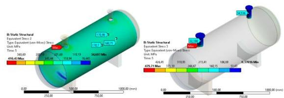
Figure 5 The state of tension in the jacket and connections
